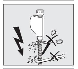
The inlet hose must **not** be shortened or damaged in any way because it contains electrical wires (see illustration).
